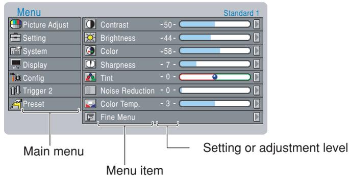
2. Use the ▲ and ▼ buttons to select a main menu (Picture Adjust, Setting, System, Display, Config, Trigger 2, Preset) and press the ► button.
