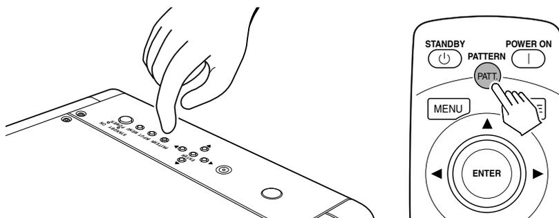
2. To focus the pattern, press the **◀ / ▶** buttons on the remote controller or projector. Tapping the buttons fine-adjusts the focus. Holding the buttons down quickly changes the focus. Adjust the focus so that the focus pattern appears its sharpest, as shown below.
