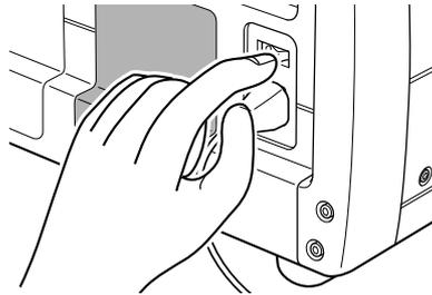
3. Press the **POWER ON** button on the remote controller or the **POWER** button on the projector. The **POWER ON** indicator on the projector will light up.
