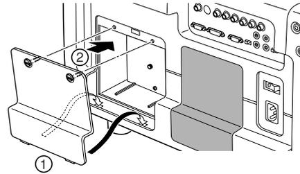
12. Lock the lamp cover in place with the 2 screws loosened in step 5. (Slotted head screwdriver required.)
