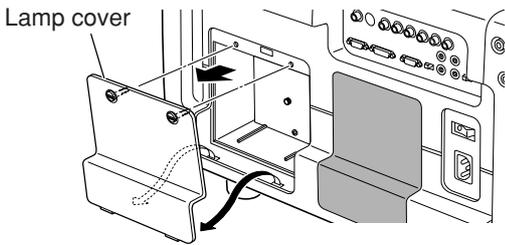
7. Remove the 2 screws that lock down the lamp shield. (Phillips screwdriver required.) Pull the lamp shield downward as indicated in the below figure and detach.
