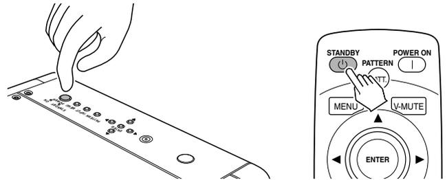
2. After the cooling fan stops, set the **ON/OFF** switch in the OFF position and unplug the AC power cable.
