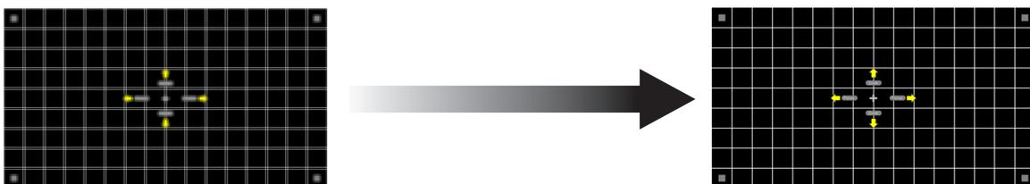
3. To adjust the size of the projected image, press the **▲ / ▼** buttons on the remote controller or projector. Tapping the buttons fine-adjusts the size. Holding the buttons down quickly changes the size.
