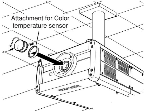
Attach the color temperature sensor so that the cable is to the bottom side of the projector (now upside-down) as shown in the figure.
