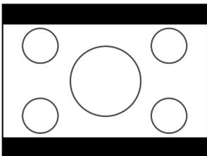
The image is enlarged to the maximum height and width of the screen, regardless of the aspect ratio of the 4:3 image.
