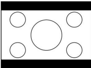
A 4:3 image is projected in the proper vertical-to-horizontal proportions.
