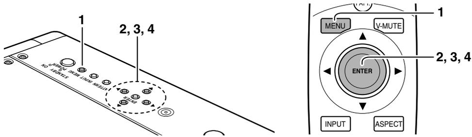
1. Press the **MENU** button on the remote controller or projector to display the menu.
