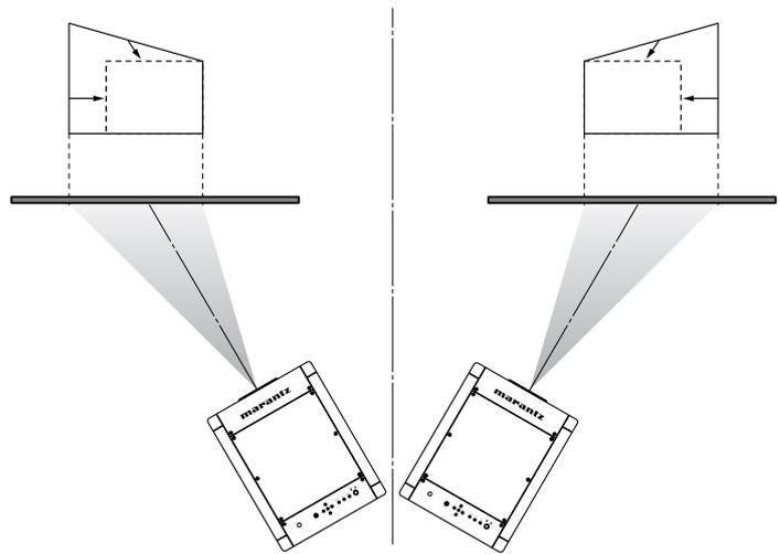
**Note :** Horizontal keystone is best corrected when the projector is installed on a flat surface and the image is shifted to the maximum height using the “Lens shift” feature in the menu.
