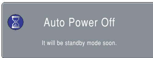
About 1 minute after the message appears on the screen, power to the projector shuts off.
