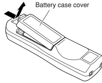
2. Insert two AA batteries with their +/- poles matching the indications inside the battery compartment.
