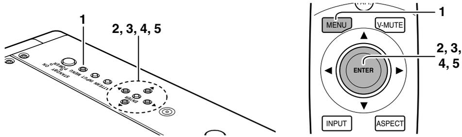
1. Press the **MENU** button on the remote controller or projector to display the menu.
